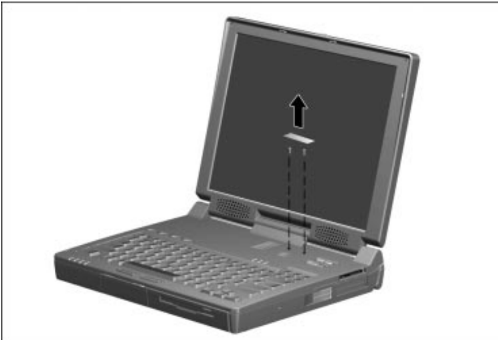
Figure 5-30. Removing the Keyboard Warning Label and Screws
