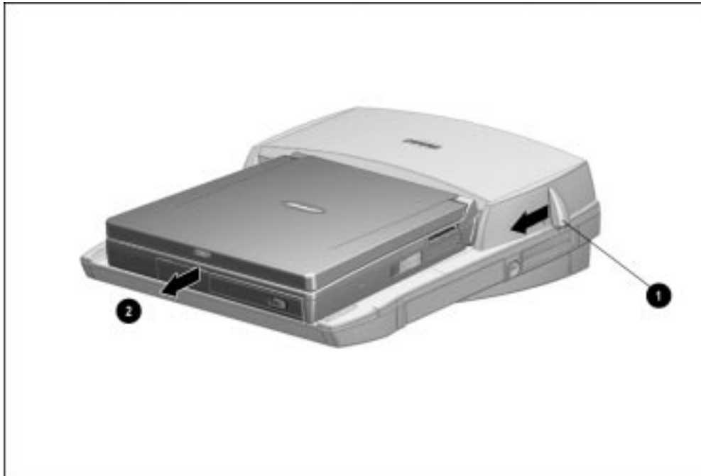
Figure 5-4. Undocking the Computer from the Armada MiniStation
