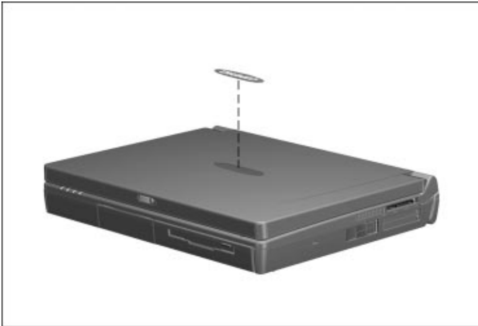
Figure 5-6. Installing the Computer Logo
