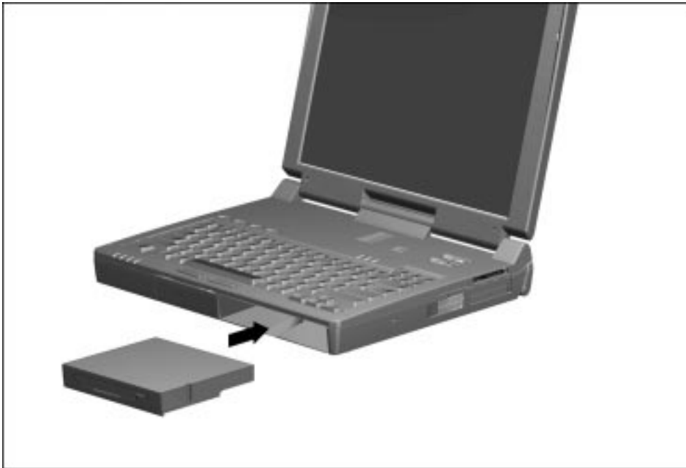
Figure 5-24. Inserting a Drive into the MultiBay
