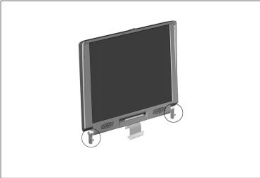
Figure 5-54. Proper Position of the Display Clutches
